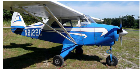
Piper PA-22 Tri-Pacer. Note-fully steerable nosewheel
